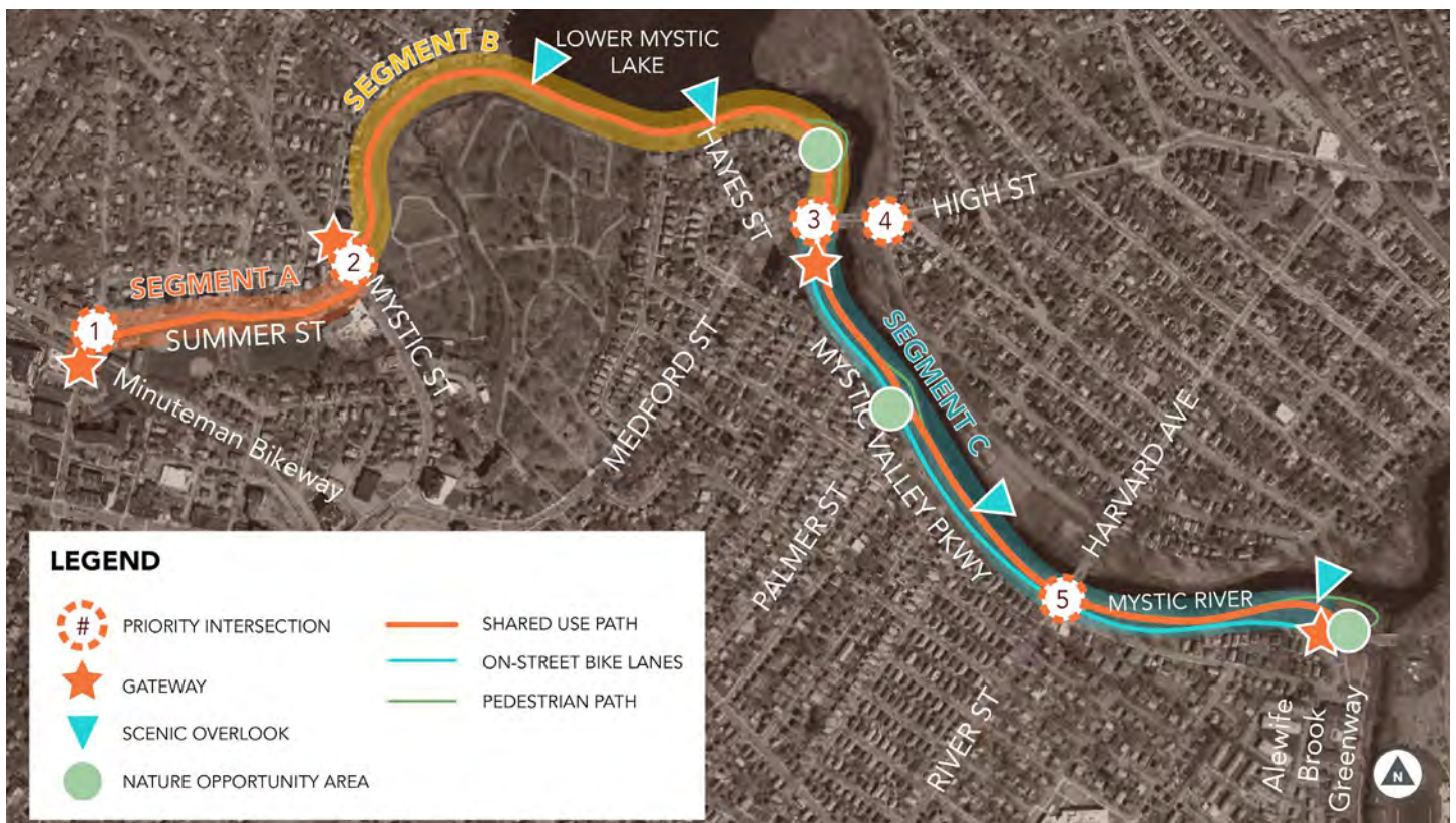
Figure 25: The recommended concept includes a continuous shared use path plus on-street bike lanes and pedestrian paths as feasible
